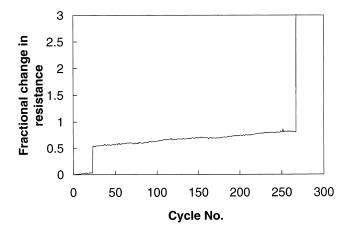
Fig. 2. Variation of the fractional contact resistance change  $(\Delta R/R_o)$  with cycle number during cyclic shear loading at a shear stress amplitude of 3.73 MPa up to bond failure.
