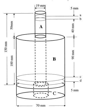
Fig. 1. Configuration for measuring contact electrical resistance during shear loading of joint between steel rebar (A) and concrete (B). Steel support (C).
