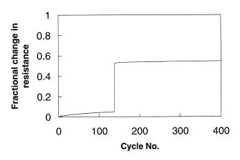
Fig. 3. Variation of the fractional contact resistance change  $(\Delta R/R_o)$  with cycle number during cyclic shear loading at a shear stress amplitude of 0.75 MPa. The test was stopped prior to bond failure.
